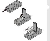
Change batteries when battery symbol is empty.
